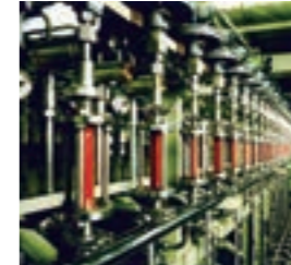
1982 Practical application of world's first RO concentration technology for concentration of tomato juice
