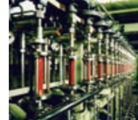
1982 Practical application of world's first RO concentration technology for concentration of tomato juice
