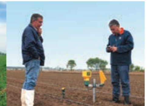
Sensors installed in fields all over the world link to satellites, collecting information such as temperature, humidity, and precipitation
